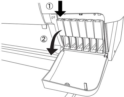
4. Carefully pull the cartridge straight out of the printer.
