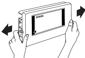
6. Hold the ink cartridge with the arrow mark on the left side and pointing to the rear of the printer. Then insert the ink cartridge into the slot. Don't force the cartridge.
