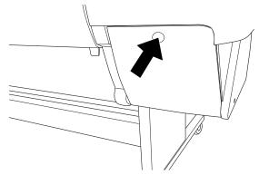
6. Hold the ink cartridge with the arrow mark on the left side and pointing toward the printer. Then insert the ink cartridge into the slot. Don't force the cartridge.
