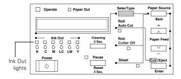
When the light stays on and INK OUT is displayed, the cartridge is empty. You must replace it before you can continue printing.
