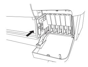
Push the cartridge clamp back up. Make sure the corresponding Ink Out light goes off. Then close the ink compartment cover.
