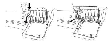
6. Insert the draining cartridge into the black ink slot. Close the ink cartridge clamp, then close the cover.
