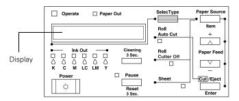
When your ink or paper runs out or a problem occurs, a message appears on the display. The lights on the control panel come on or flash. The following table lists the messages and includes an explanation and instructions for correcting the problem.
