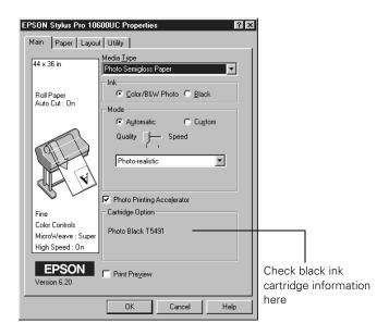
If necessary, set the information manually. Click the Utility tab, then click the Printer and Option Information button. Select the appropriate ink cartridge option, as shown below.
