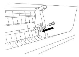
9. Push down on the cutter's side pin while turning the latch to the left.
