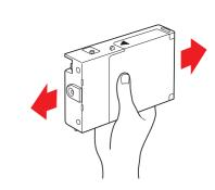
Install the ink cartridges in the printer. Hold each cartridge with the arrow pointing toward the printer, then insert it into its slot. Make sure you insert each cartridge in the correct slot.
