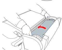
Feed the paper all the way through the printer until it is aligned with the OTHERS mark on the paper tray cover. Align the right edge with the vertical mark on the right side of the tray cover. Then return the paper lever to the secured position and close the roll paper cover.
