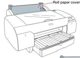
6 Place the paper and spindle in the printer as shown, with the black end on the left.
