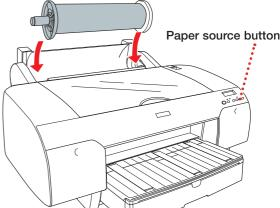
Make sure the printer is powered on and ready. Press the ≤ paper source button until the 🦭 🐰 or noll paper icon appears.
