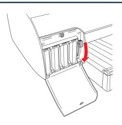
When **READY** appears on the LCD display, charging is complete. Close the ink compartment covers.
