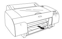
4. If you can't reach the paper from the front, remove it from the back of the printer.
