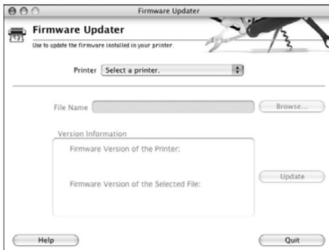
6. Make sure your printer is on, its LCD is set to Ready, and it is connected to your computer, then choose Stylus Pro 4800 in the Printer list.
