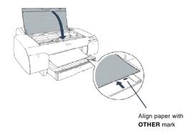
**7** Return the paper lever to the secured position. The printer grabs the paper and feeds it into printing position.
