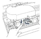
**6** Release the side pin and carefully remove the cutter blade.
