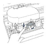
**9** Close the top cover. The carriage returns to the home position and the cutter replacement is complete.
