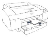
**7** Flip down the paper guide roller, then replace the paper tray cover and adjust its length.
