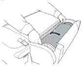
**9** Make sure the paper is aligned with the **OTHER** mark and the vertical line next to the arrow. Then return the paper lever to the secured position.
