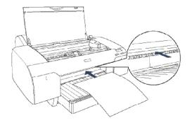
**5** Push the sheet under the gray feed rollers, and align the right edge with the vertical mark on the right side of the tray cover.
