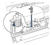
**8** Hold down its side pin and secure it with the latch.
