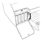
**7** If you're using 110 ml cartridges, close the ink compartment cover. If you're using 220 ml cartridges, you'll have to leave the cover open.
