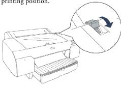
**8** Extend the paper tray and cover to support the sheet as it comes out of the printer. Make sure the roll paper support is not raised.
