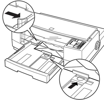
4. Adjust the rear and left edge guides as shown above so the media feeds straight into the paper path.
