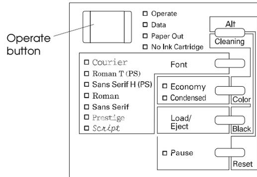
Since most printer settings can be controlled from software, you do not often need to use the control panel. This section describes how to read the lights and the buttons on the control panel.
