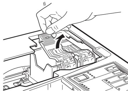
5. Lift the cartridge out of the printer and dispose of it carefully so any excess ink does not spill. Do not take the used cartridge apart or try to refill it.
