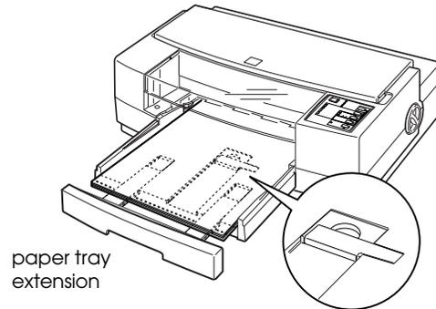
3. Gently pull the extension out using both hands—one to hold the paper tray in position and the other to pull out the extension.
