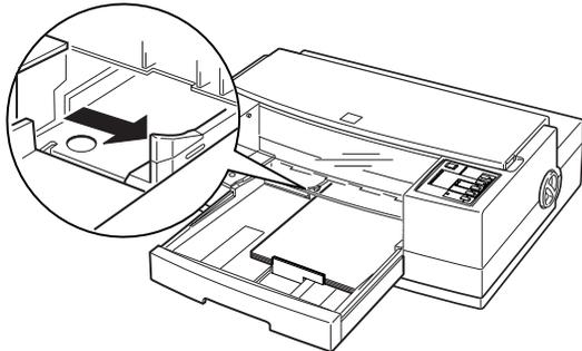
You can load up to 100 sheets of plain bond paper, but do not load paper above the arrow mark on the left edge guide.
