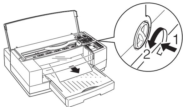
Be sure to turn the knob in the direction shown; otherwise ink from the printed sheet can come off on the printer and smear other sheets.
