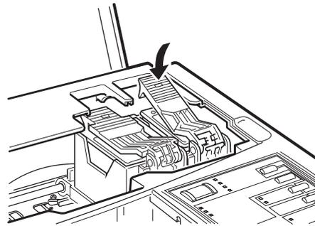
9. Clean the print heads to ensure that ink is properly delivered to each nozzle. Cleaning is recommended but not required.
