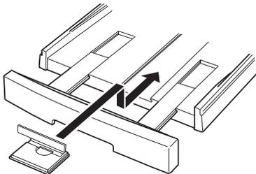
3. Insert the paper or envelopes into the paper tray. It is best to load sheets of heavy paper one at a time. If you're loading envelopes, insert them as shown. You can load up to 10 envelopes.
