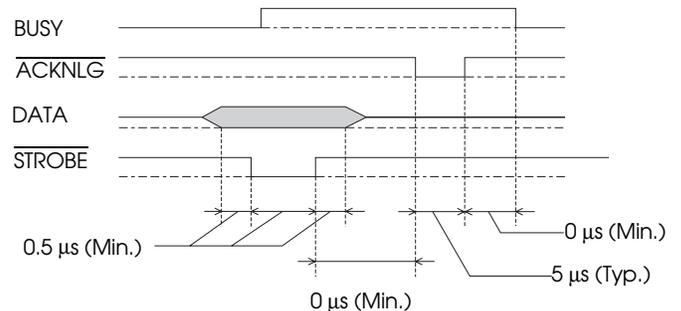
Transition time (both the rise and the fall) of every signal must be less than 0.2  $\mu$ s.
