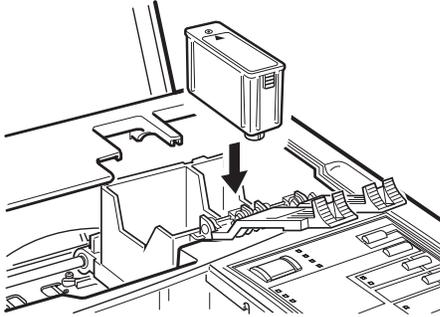
Be sure to install both ink cartridges. The printer will not work if only one cartridge is installed.
