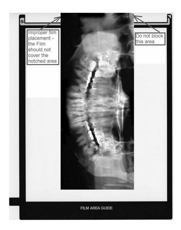
The image below is an example of the final scan when the film is not correctly placed on the bed. The film was placed in the area where the scanner takes a white calibration reading. Note the very light "washed out" areas and lines throughout the scan.
