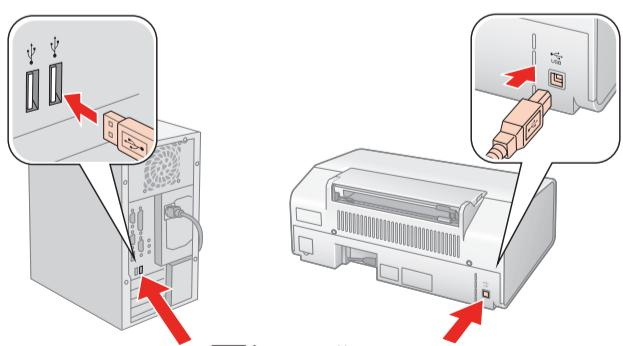
**Note:** If installation doesn't continue after a moment, make sure you securely connected and turned on the R280 Series.
