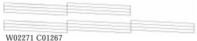
Each staggered horizontal and straight vertical line should be complete, with no gaps in the dot pattern. If your printout looks okay, you're done. If any dots are missing, clean the print heads again, as explained in the previous sections.
