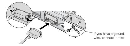
3. Connect the other end of the cable to your computer's parallel port and secure it as necessary. See your computer documentation for details.
