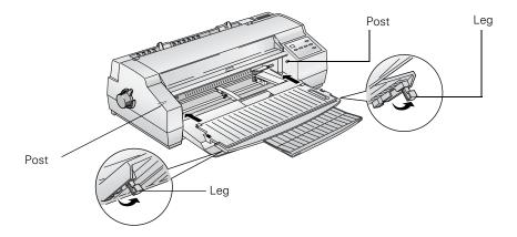
3. Flip down the legs on the underside of the output tray so it sits up on the paper support.
