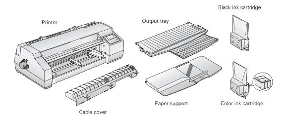
Place the printer flat on a stable desk near a grounded outlet. Leave plenty of room in back for the cables and for a stack of continuous paper, if you use it. Leave enough room in front for the paper support and output tray.
