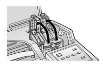
4. Lower the ink cartridges into their holders with the labels face up and the arrows pointing toward the back of the printer.
