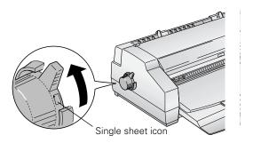
2. Lock the output tray in an upright position on the two upper posts.
