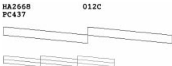
Each staggered horizontal and straight vertical line should be complete, with no gaps in the dot pattern. If your printout looks okay, you're done. If any dots are missing, clean the print heads again, as explained in the previous sections.
