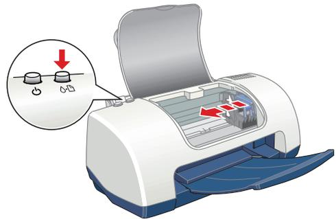
3. Pull up the ink cartridge clamp and remove the cartridge. Dispose of it carefully.
