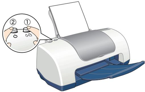
4. Turn off the printer after it prints the check page. Then reconnect the cable and turn on your printer and computer.
