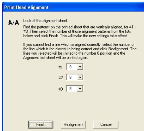
5. Click **Realignment** to print another test page. Make sure the pattern numbered 8 in each row is the best aligned. If not, repeat steps 4 and 5.
