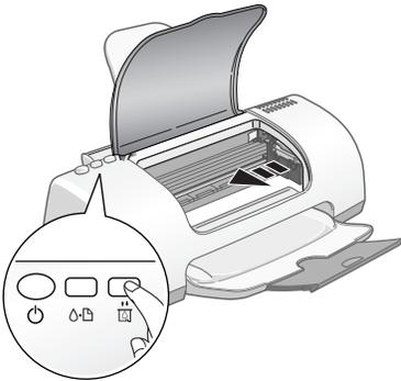
2. Lift up the ink cartridge clamp. The cartridge rises up from its holder.
