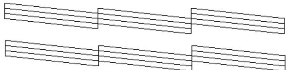
Each staggered horizontal and straight vertical line should be complete, with no gaps in the dot pattern. If your printout looks okay, you're done. If any dots are missing, as shown below, clean the print head again; see "Cleaning the Print Head" on page 14 for instructions.
