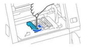
**5** Lift and remove the front side of the cap.
