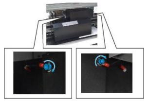
**10** Tighten the four screws on the front of the printhead.
