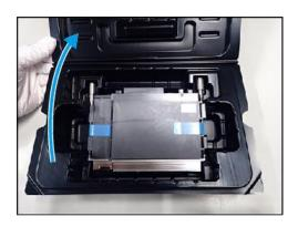
2 Insert your finger into the recess next to the printhead and remove the printhead.
