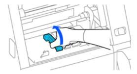
6 Put the used cap in the bag that contained the new cap to prevent ink from getting around.
