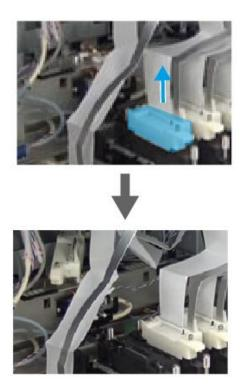
**13** Completely loosen the two fixing screws on the printhead.
