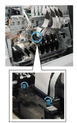
**12** Pull the connector straight out and put it in the back.
