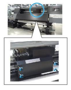
**8** Remove the two screws on the upper left and right sides.
