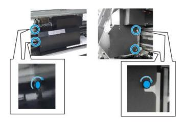
**9** Tighten the two screws on the top of the left and right sides after attaching the Y-type terminal.
