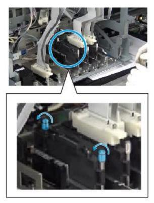
**14** Hold the head of the screw and pull the printhead straight up.
