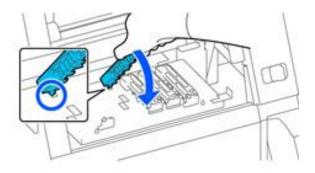
3 Install and tighten the screw in front of the cap.
