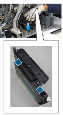
4 Tighten the fixing screw firmly.
