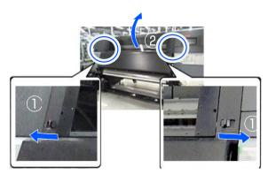
**7** Remove the four screws on the front of the printhead.
