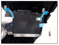
4 Replace the printhead in the protective case.
