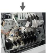
**11** Completely loosen the two screws on the connector at the top of the printhead.
