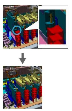
Make sure that the protrusion fits into the positioning hole at the bottom of the print head when you insert it all the way down.
