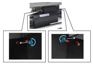
**9** Loosen the 4 screws on the left and right sides by 3 turns.
