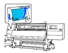
4 Loosen the screw in front of the cap with a Phillips screwdriver and remove it.
