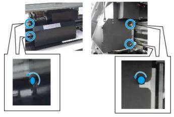
**10** Lift the printhead cover slightly and remove it toward you.
