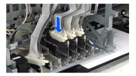
**6** Tighten the connector screws.
