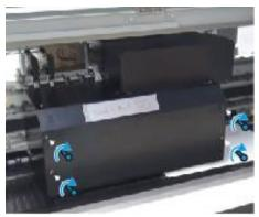
**11** Close the front cover and move the left and right lock levers inward.
