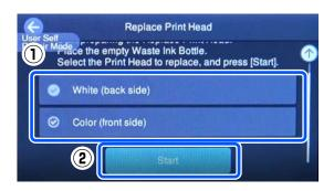
The oicon indicates the Print Head that is selected to be replaced. (In the illustration above, the **Color (front side)** is to be replaced.)
