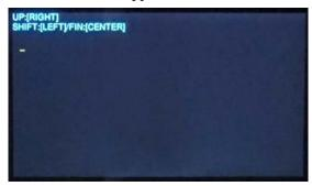
If the screen in the illustration does not appear, and the power just comes on as normal, turn off the power and redo the procedure from step 2.
