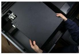
After removing the cover, place it on the top of the Printer Cover with the inside facing upward.
