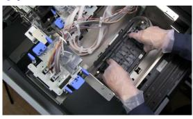
Place the used Print Head that you removed on the lid of the protective case.
