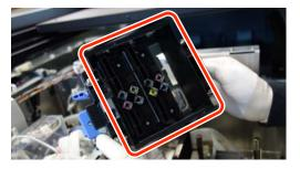
Lightly press on the handles of the Ink Damper Unit to assure it is installed.
