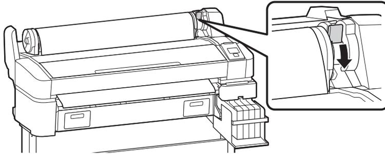
11. Following the instructions on the control panel, press the OK button. The paper will be fed into the printer.
