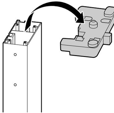
5. Fasten the mounting piece to the bracket using two B screws.
