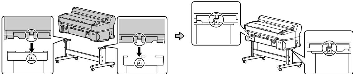
4. Attach the printer to the stand using three A screws.
