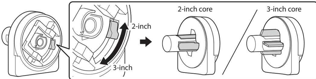
4. Raise the adapter lock lever to release the lock on each of the two roll paper adapters.
