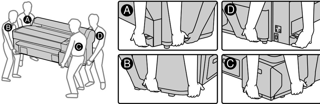
**Caution:** When lifting the printer, only hold the highlighted areas, otherwise the printer may not operate or print normally.
