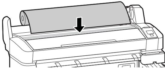
3. If necessary, adjust the Roll paper adapters to fit the core size of the roll paper.
