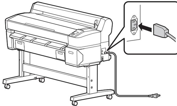
7. Plug the power cord into a properly grounded electrical outlet.
