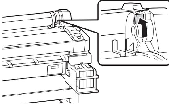
2. Place the roll paper on top of the printer.
