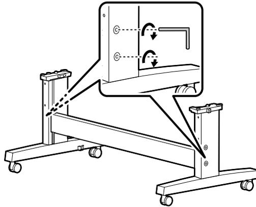
3. Remove the four screws as shown.
