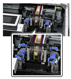
Lift up the Ink Damper Unit and hang it temporarily on the hook.
