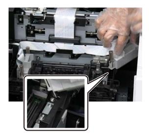
Remove the left side connector in the same way, and place it on the holder.
