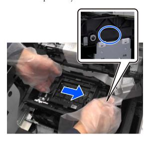
While holding the parts shown in the photo, press down on the Print Head and rotate it slightly clockwise.
