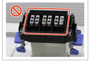
Use your fingers to turn the connector fixing screws (4 pc) counterclockwise to loosen them.
