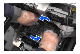
While holding the right side of the carriage to prevent it from moving, push the Print Head to the right.
