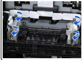
Hold the Ink Damper Unit with both hands and gently push it down to remove it from the temporary placement hook.
