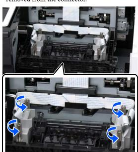
Lift the right side connector straight up to remove it, and place it on the holder.
