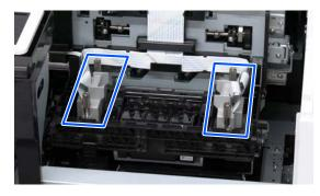
Use your fingers to turn the fixing screws (4 pc) clockwise to secure the connector.
