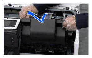
9 Lift the temporary placement hook on the maintenance cover.
