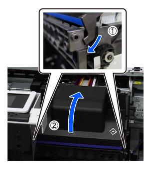
Hand-tighten the screw on the carriage cover.
