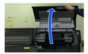
Squeeze the lock on the carriage cover to unlock it, and then open the carriage cover towards you.
