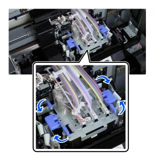
Lift up the Ink Damper Unit and hang it temporarily on the hook.
