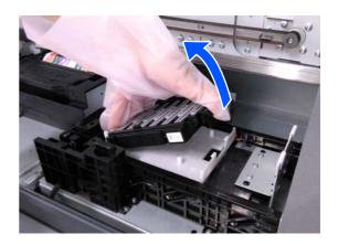
Put the removed anti-drying caps in the bag that contained the new ones.
