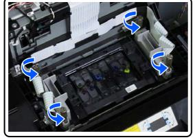
Lift the right side connector straight up to remove it, and place it on the holder.
