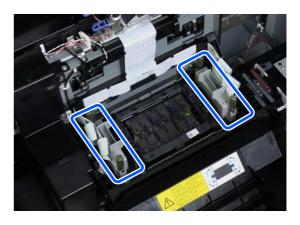
Use your fingers to turn the fixing screws (4 pc) clockwise to secure the connector.
