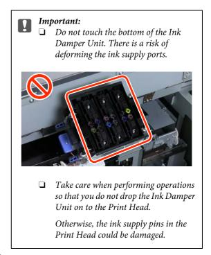
Lightly press on the handles of the Ink Damper Unit to assure it is installed.
