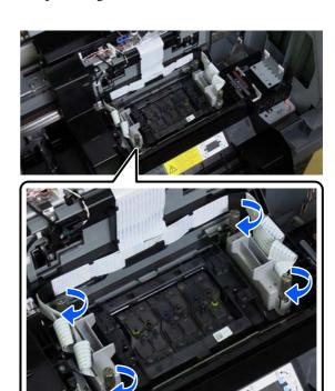
Hold the Ink Damper Unit in both hands, and install it on the Print Head.
