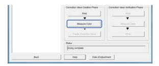
When the screen is displayed, check that the light on the right of the color measurement device is flashing green, and then insert the correction chart that matches the color chart ID and preset ID displayed on the screen into the color measurement device.
