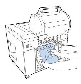
Remove the Cleaning Sheet from the rear roll paper feeder after a warning buzzer sounds indicating that cleaning is complete. Finally, install the Spindle unit for the rear roll paper feeder as it was before.
