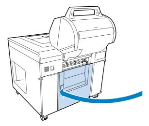
For the Dual Roll Model, press the front roll paper feeder down as far as it will go.
