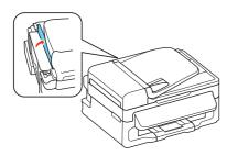
**2** Raise the paper support, pull out the output tray, then raise the paper stopper.
