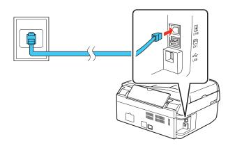
**Note:** If you're connecting to a DSL phone line, you must use a DSL filter or you won't be able to fax. Contact your DSL provider for the necessary filter.
