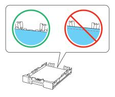
Slide the edge guides against the paper, but not too tight. Make sure the paper is under the tabs on the edge guides.
