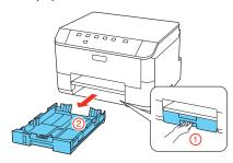
2 Slide the edge guides outward, and position them for the type of paper you are using.
