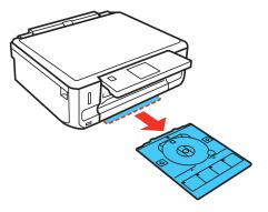
9. Place a CD or DVD on the CD/DVD tray with the printable side faceup, and insert the tray into the slot above the output tray.
