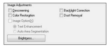
**Note:** Select the **Image Option** checkbox if you need to set any of the grayed-out image adjustments. Not all adjustment settings may be available, depending on the Document Type and Image Type setting. Click the **Brightness** button to access additional settings.
