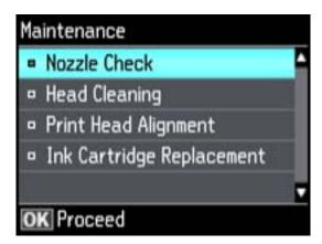
6. Press the arrow buttons to select **Print Head Alignment**, then press **OK**.
