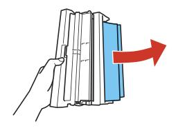
4. Open the duplexer and remove any jammed paper from inside it.
