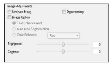
**Note:** Select the **Image Option** checkbox if you need to set any of the grayed-out image adjustments. Not all adjustment settings may be available, depending on the Image Type setting.
